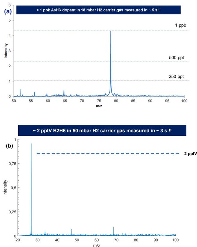
Fig. 4. iTrap® Mass spectrum showing (a) sub-ppbV level of  $\text{AsH}_3$  and (b) single-digit pptV  $\text{B}_2\text{H}_6$  in  $\text{H}_2$  carrier gas flow. The measuring time was around 3 to 5 sec. The spectra were recorded in the so-called one-short mode where no signal averaging nor integration were applied.
