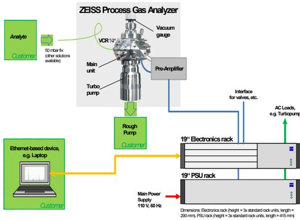
Fig. 1. Schematic drawing of the iTrap® system of Carl Zeiss SMT GmbH together with its peripheries.
