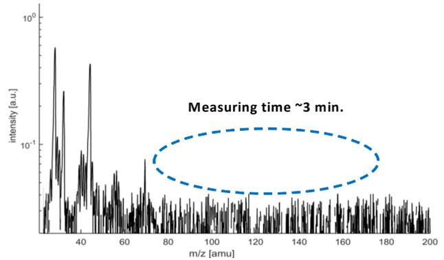
Fig. 3(a). RGA mass spectrum of organic outgassing of a photo-resist plus a lubricant-contaminated O-ring. Signals from the contaminated O-ring (above 80 amu) was missing due to mass discrimination with increasing m/z-ratio in RGA. Measuring time for the entire spectrum was around 3 minutes.
